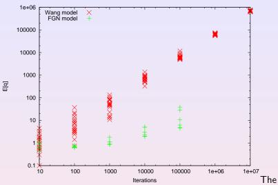
effect of increasing the number of iterations on  $\mathsf{E}\left[q\right]$  in two LRD models.
