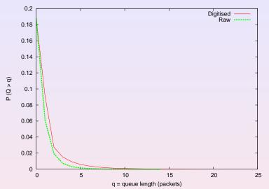
1 - PDF of queue size in packets before and after digitisation of the Bellcore data (queued at half bw).
