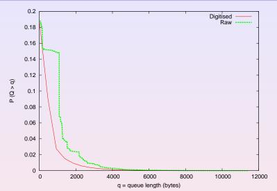
1 - PDF of queue size in bits before and after digitisation of the Bellcore data (queued at half bw).
