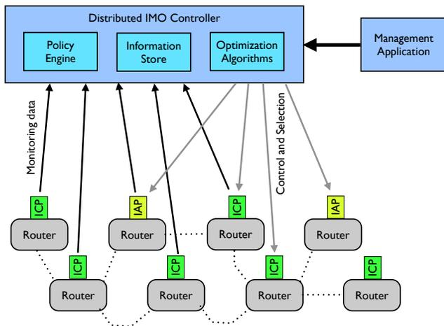
Fig. 1. Information Management Overlay (IMO) Controller and Routers
